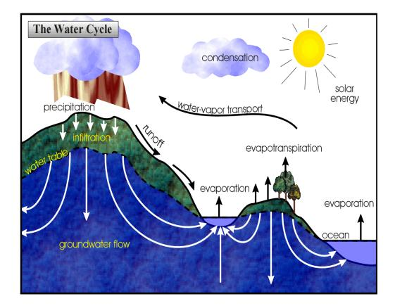
Surface water is precipitation that does not soak into the ground, but runs off into streams, ponds, lakes, and rivers. Watersheds are the catch basins for all precipitation falling from the sky, and rain or snow falling within the confines of a watershed's interconnected high points eventually becomes surface and groundwater.
