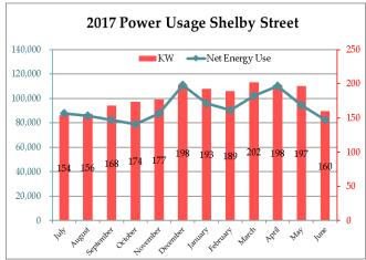
The energy usage (KW) follows the peak flows in the sewers; this is a measure of the success of the City's program to reduce Inflow and Infiltration into the Sewer System. Weather drives our Flows and Autumn through Spring proved wetter than last fiscal year.
