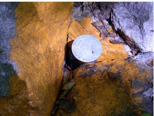
The DRED Easement corner pins are well marked and easy to find.
